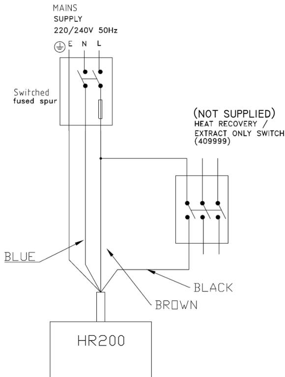
1. Wiring must be via a 3A fused switched spur with a 3mm contact separation in each pole. The wiring should be suitably (Basec or Har) approved cable of appropriate current carrying capacity.
